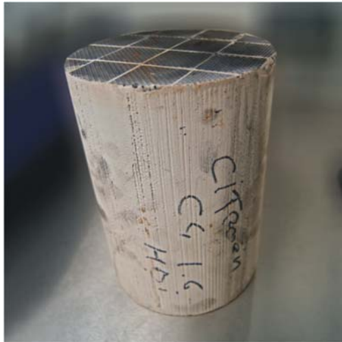
Figure 2: A built-out (closed) ceramic filter element, used in a Citroen C4. This particle filter has a diameter of about 10 cm and is about 20 cm high (photo: TNO at Digicar Engineering).
