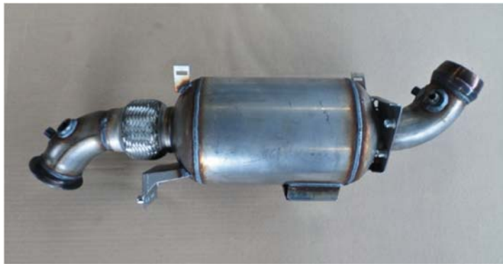
Figure 1: Diesel Particle Filter of a passenger vehicle, as part of the exhaust system. The filter element (see Figure 2) is in the metal housing (photo: Topcats)
