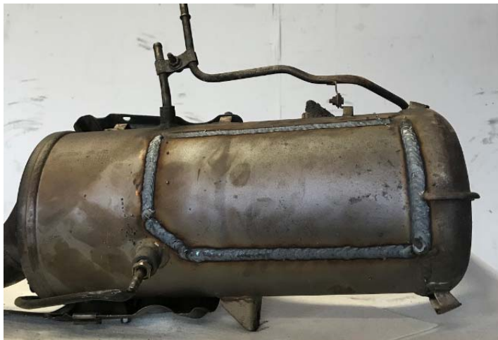
Figure 3: Internally adjusted Diesel Particle Filter (photo: OBD-Chiptuning).
